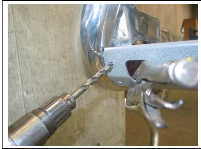
Figure 13: Drill out lower protection plate to 5/16 (8mm)
