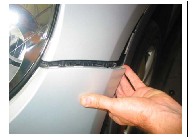
Figure 2: Pull bumper out from guard, then forward
