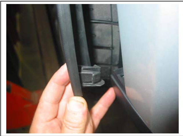
Figure 1: Plastic clip on rear of guard trim
