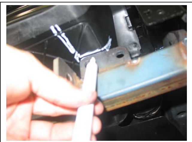
Figure 5: Mark underside of air dam for trim
