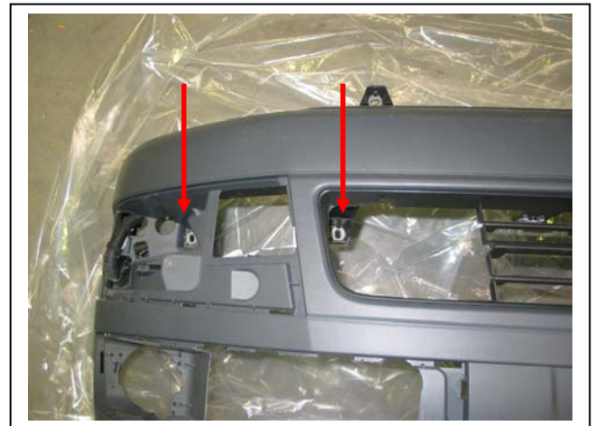
Figure 4: Remove two T25 Torx screws. Photo shown with cut outs for ease of view.
