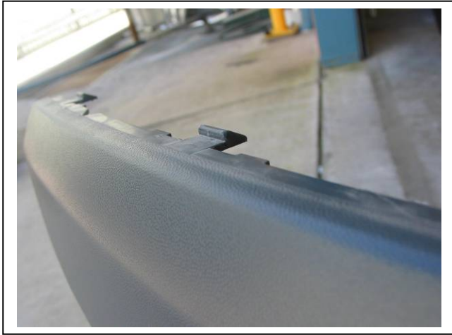
Figure 1: Bumper side panel holding clips. Passengers side shown.
