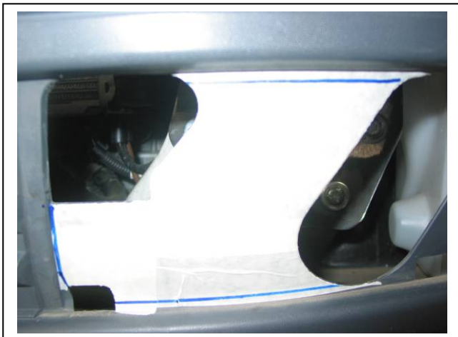
Figure 9: Remove marked section from plastic bumper cover.
