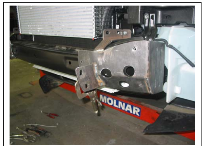
Figure 6: Chassis mount attached to vehicle. Passengers side shown.
