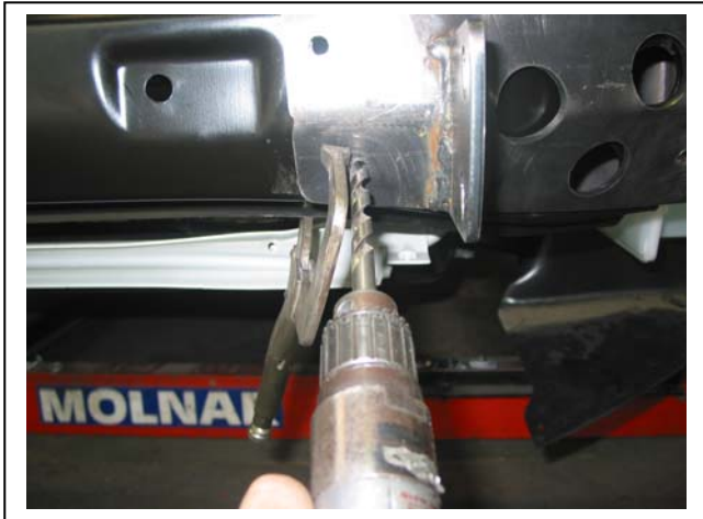
Figure 7: Drill lower inner to 10mm
