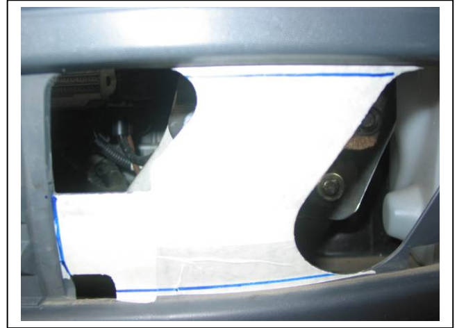
Figure 9: remove marked section from plastic bumper cover.
