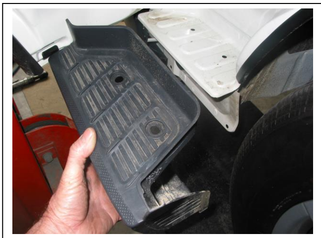
Figure 1 – Shown removing passenger side step infill
