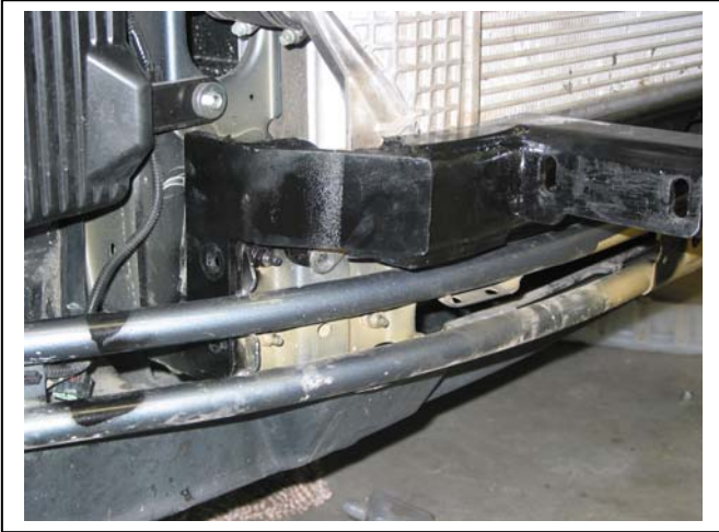
Figure 3 – Placing steel mounting bracket, ready for installation, Turbo diesel vehicle shown.
