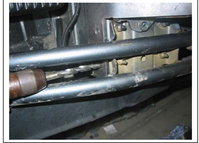
Figure 4 – Driver's side shown. Use long 10mm drill bit as required.
