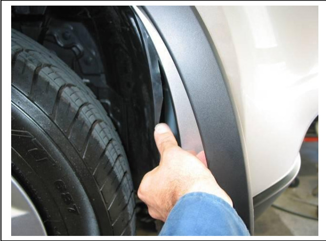
Figure 1 – View of Flare, removed from guard
