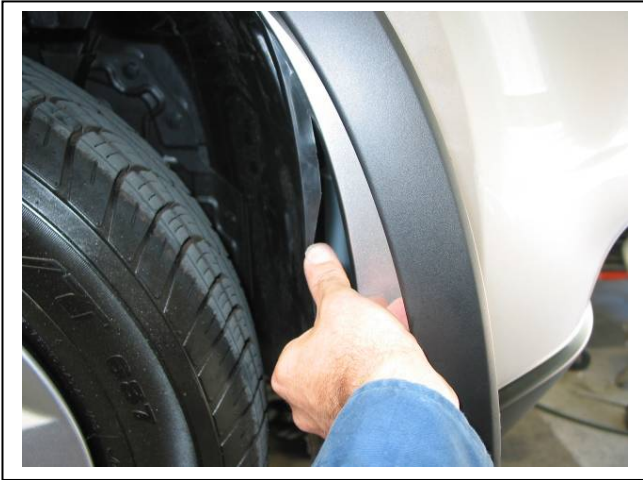
Figure 1 – View of Flare, removed from guard
