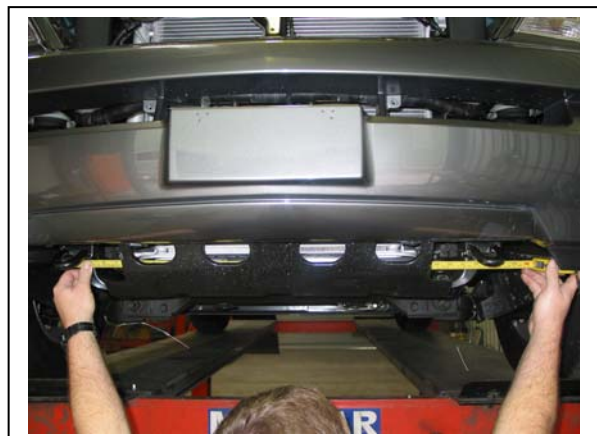
Figure 6 Checking steel angle mounts distance apart
