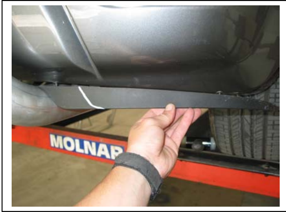
Figure 7: Chin spoiler trim, passenger side shown
