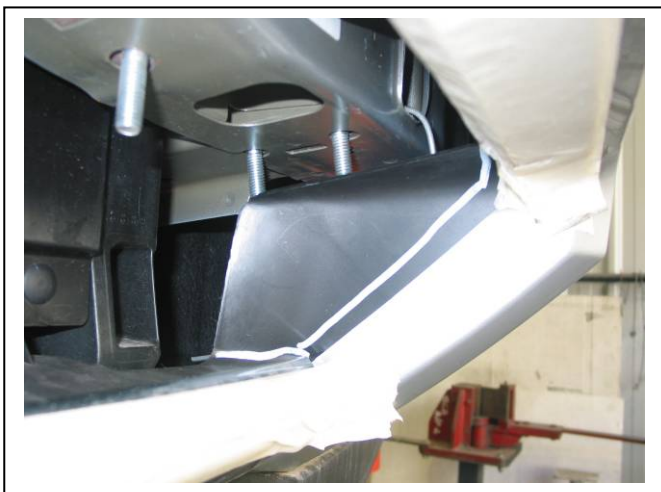
Figure 1 – Passengers side lower vent shown ready marked for cut
