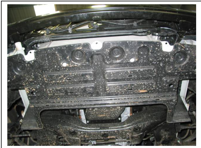
Figure 1: Front under body guard showing front four 10mm head bolts.
