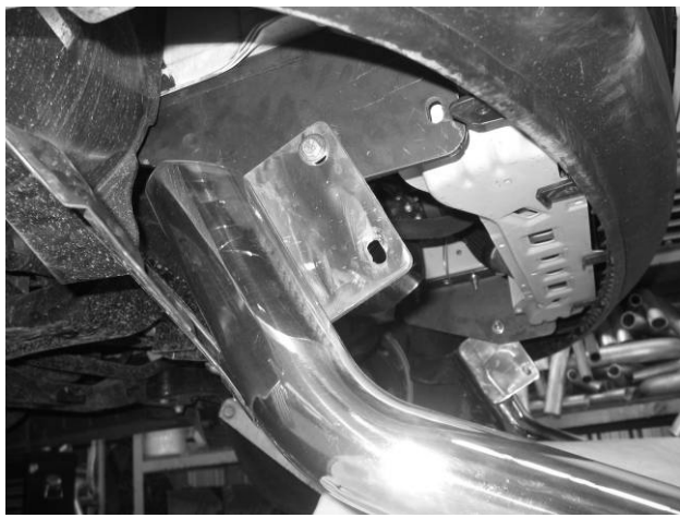
Figure 5: Rear bolts installed before Nudge Bar swung up onto vehicle.
