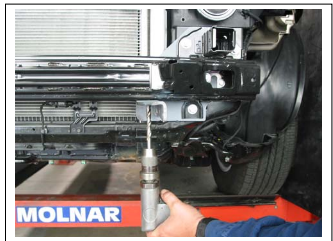
Figure 4 Drill passenger side cross member. Start with small pilot hole
