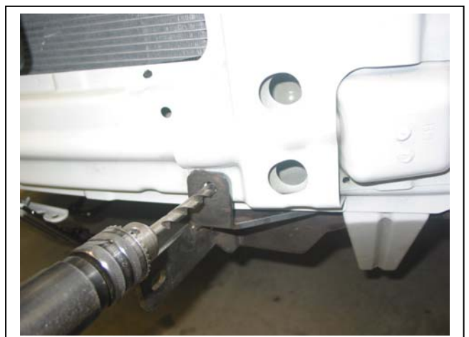
Figure 2: Remove four bolts (per side) from front of chassis rail.
