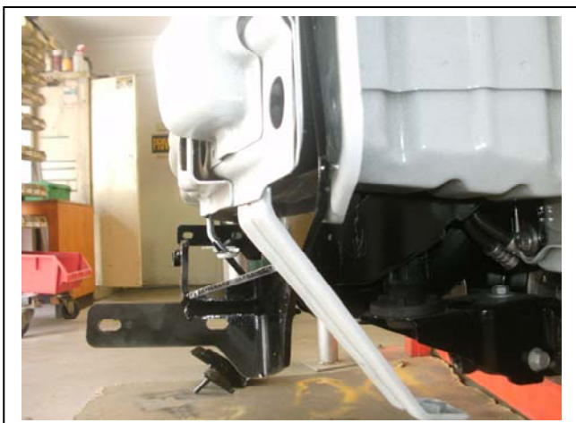
Figure 1: Carefully pull out side of bumper, unclipping from guard clips.
