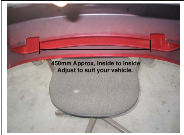
Figure 7 – View from top inner of completed trim.
