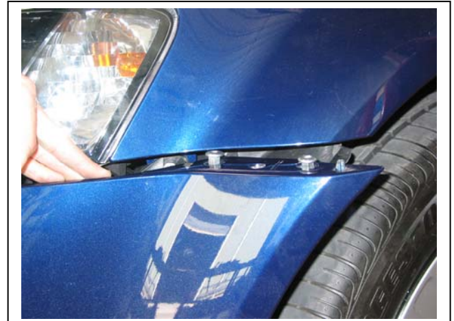
Figure 8 – Passenger side shown. Loosely fit original nuts and bolts to make it easier to refit bumper cover.
