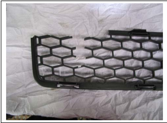
Figure 7: Grille trim to match bumper cut out
