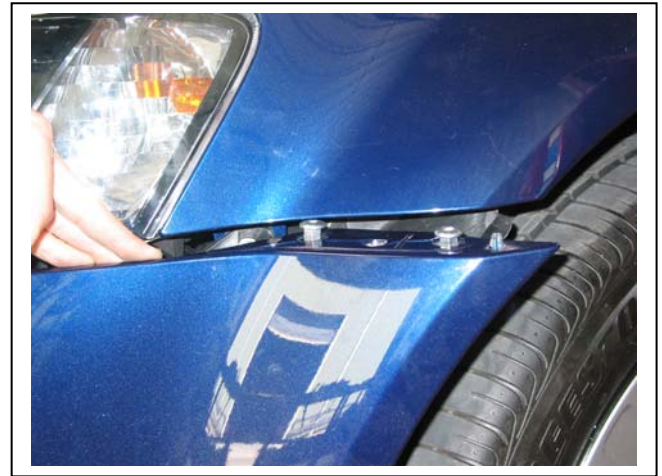
Figure 7 – Passenger side shown. Loosely fit original nuts and bolts to make it easier to refit bumper cover.
