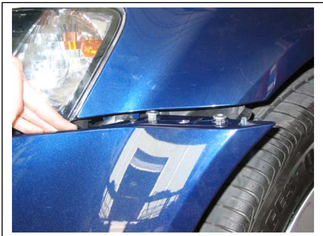
Figure 7 – Passenger side shown. Loosely fit original nuts and bolts to make it easier to refit bumper cover.
