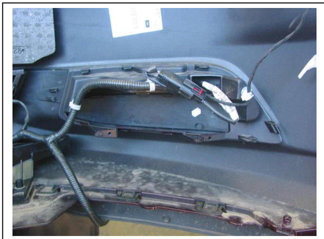
Figure 5 – Parking sensor wiring before movement
