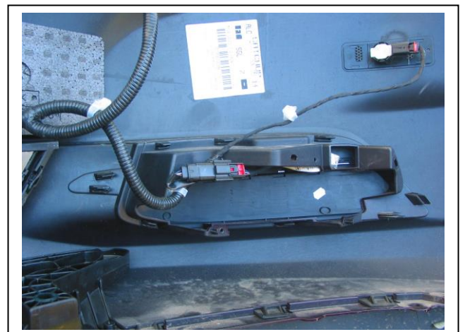
Figure 6 – Parking sensor wiring after movement
