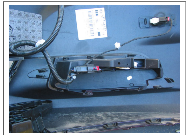
Figure 6 – Parking sensor wiring after movement
