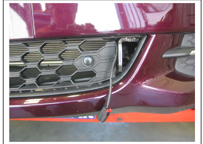
Figure 8 – Mounts shown bumper fitted
