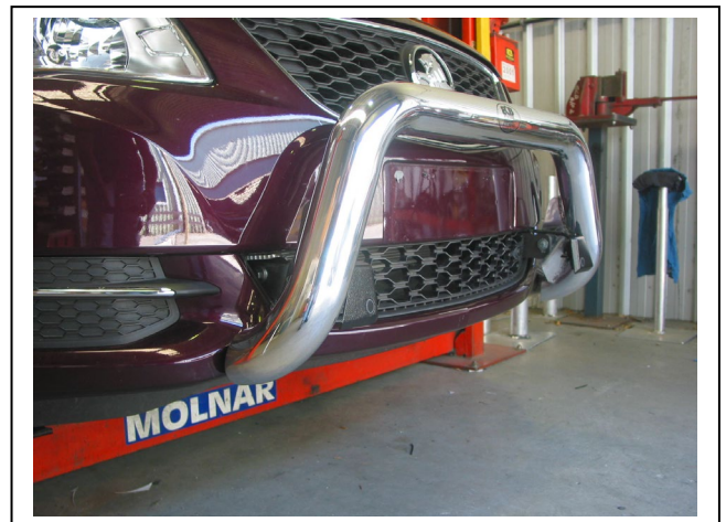
Figure 12 – Protection bar with sensors fitted
