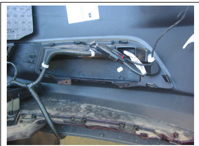
Figure 5 – Parking sensor wiring before movement
