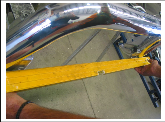
Figure 13 – sensors parallel to front face of ECB Protection bar
