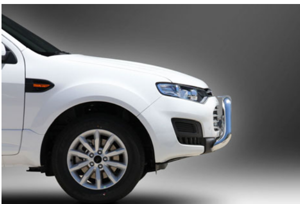
Figure 7: 76mm Nudge Bar front view
