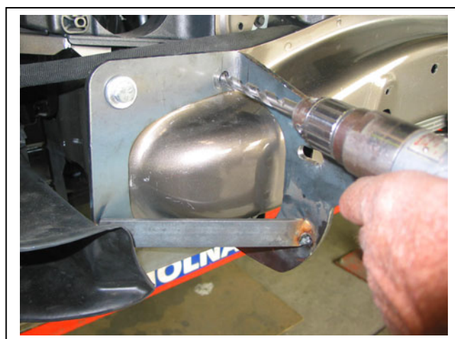
Figure 2: Drill four holes to 10mm (per side)
