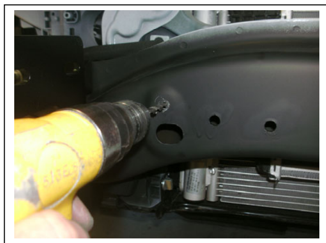
Figure 4: Enlarge one hole per side for polystyrene foam bumper support
