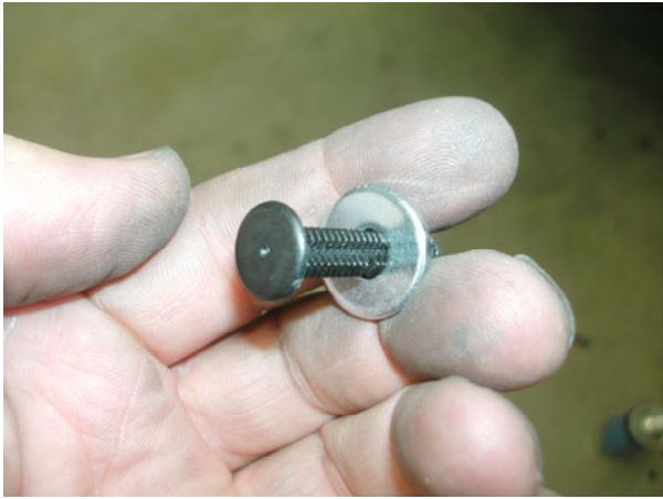
Figure 5: Place M6 washer over Christmas tree plug to enlarge size of head.
