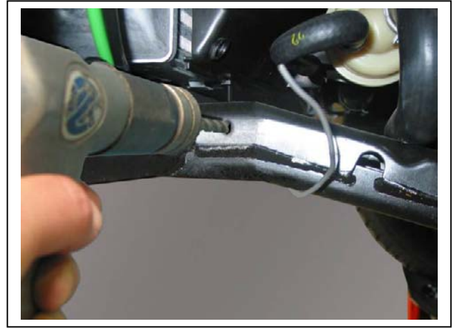
Figure 2: Drill lower front hole of engine side cover to 10mm
