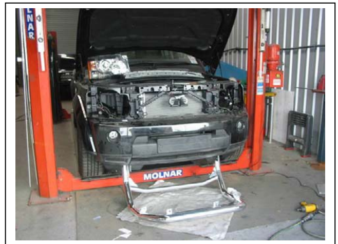
Figure 4: A soft blanket or towel will leave less marking on a mirror polished finish
