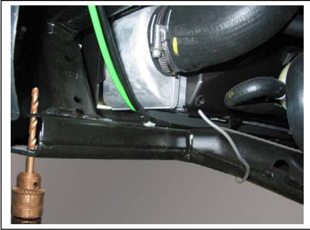
Figure 1: Drill end of lower cross member through top using lower hole as a guide
