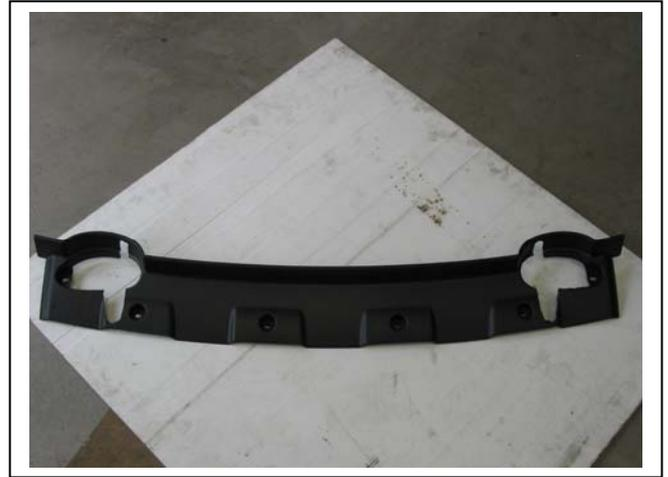
Figure 6 – Trim driver's side to match original passenger side cut out
