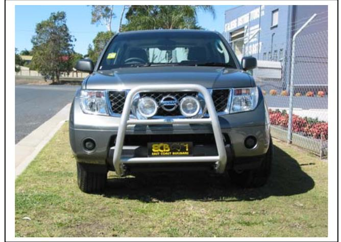
Figure 12 – 63mm Series 2 Nudge Bar front view shown
