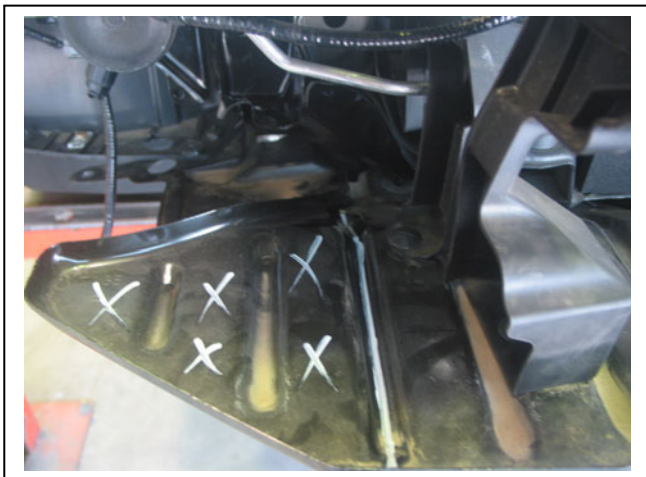
Figure 5 – Steel splash guard trim mark out.
