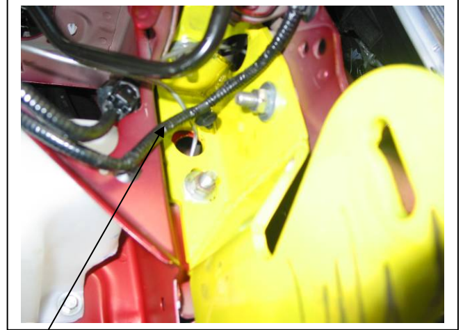
Wiring removed and relocated with mount fitted
