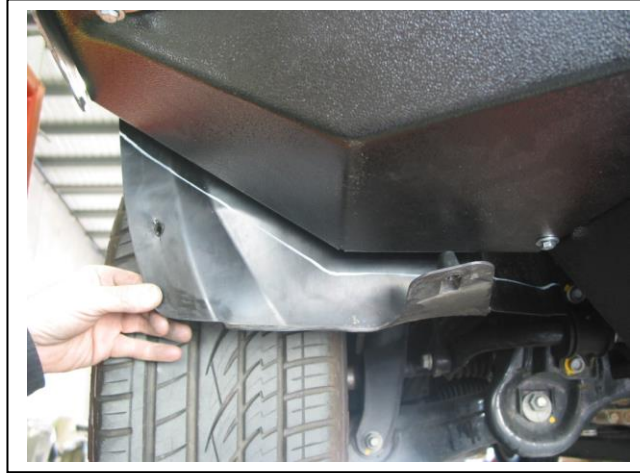
Figure 23: Cut line for inner guard. Attach using three self tapping screws.
