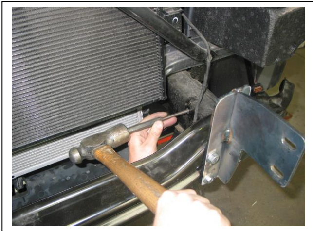
Figure 1: Remove riveted nut (nutsert)
