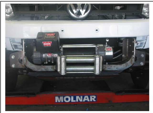
Figure 7: Warn XP9.5 fitted to winch frame.
