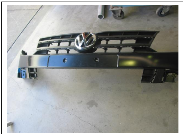
Figure 9: Centre of grille cut at top and removed.
