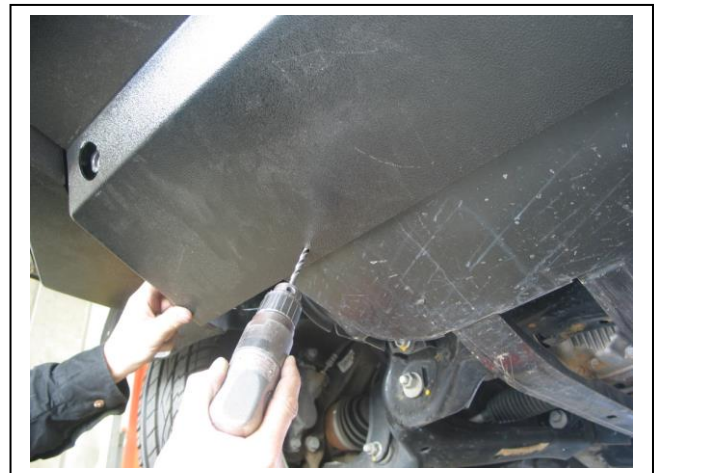
Figure 22: Drill underbody guard hole to 6mm
