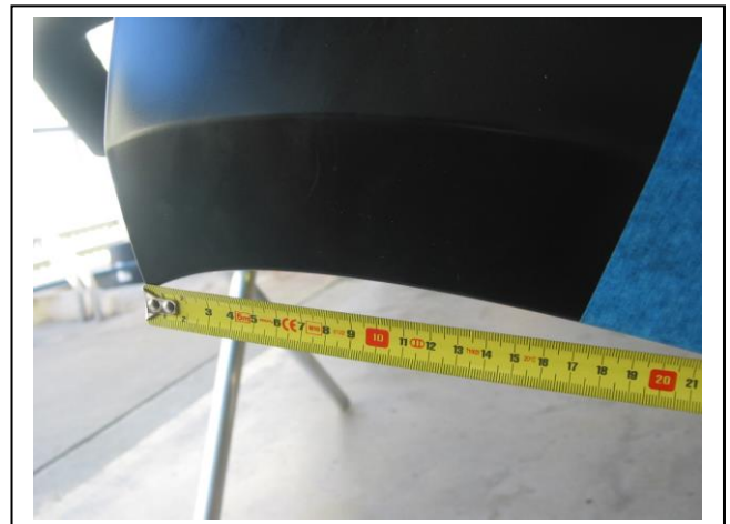
Figure 8: Measure rear of plastic bumper 220mm to cut line on bumper.
