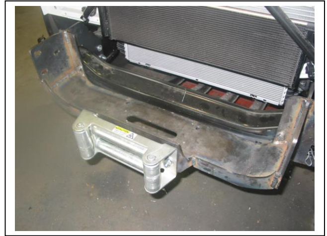
Figure 6: Fairlead roller fitted to winch frame. Finger tighten only
