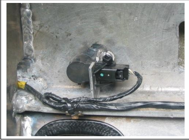
Figure 17: Parking sensor finish mounted.
