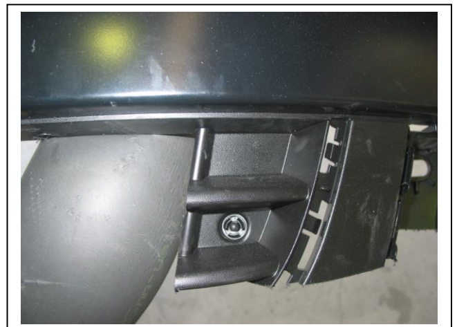
Figure 10: Cut side of grille under second rib. Retain thermo sensor mounting point.
