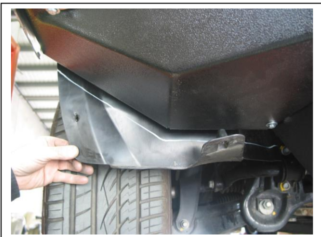
Figure 21: Cut line for inner guard. Attach using three self tapping screws.
