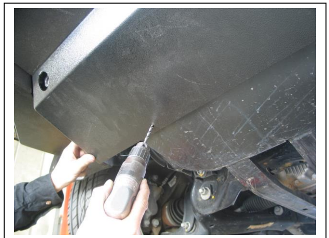
Figure 20: Drill underbody guard hole to 6mm
