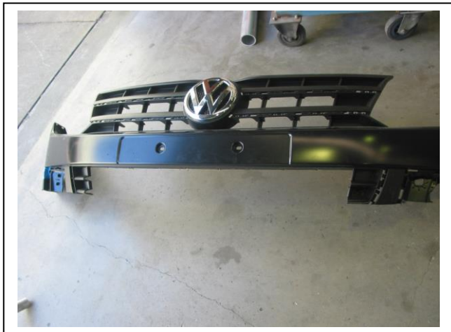
Figure 7: Centre of grille cut at top and removed.
