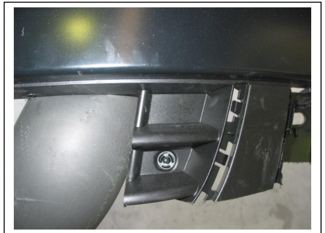
Figure 8: Cut side of grille under second rib. Retain thermo sensor mounting point.
