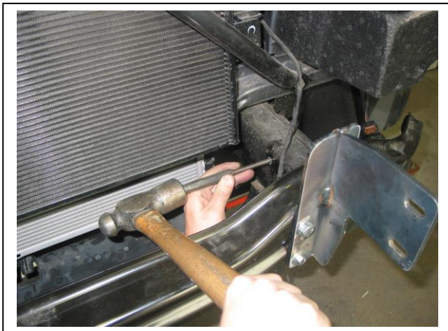
Figure 1: Remove riveted nut (nutsert)
