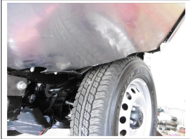
Figure 14. Liner trimmed to fit
