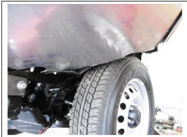
Figure 17. Liner trimmed to fit
