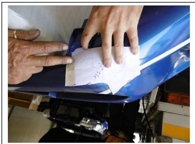
Figure 17. Liner trimmed to fit
