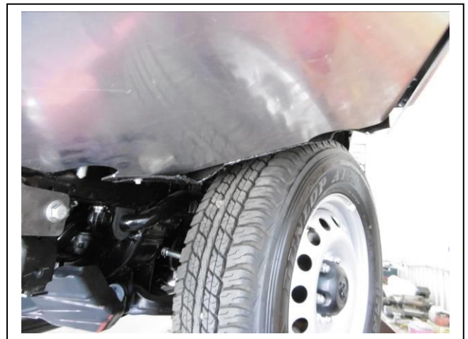
Figure 14. Liner trimmed to fit
