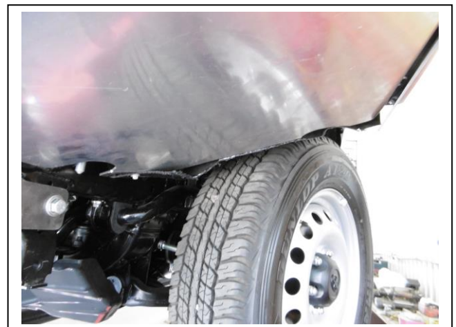
Figure 20. Liner trimmed to fit
