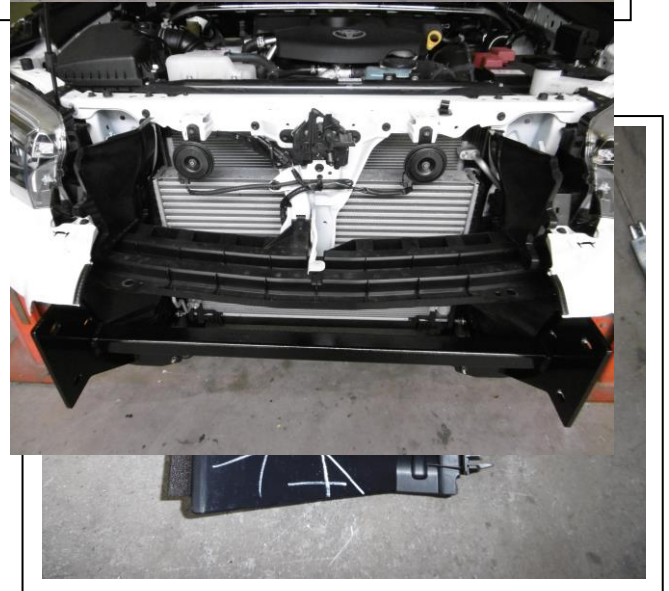
Figure 6. Trim air dam to fit around winch cradle
