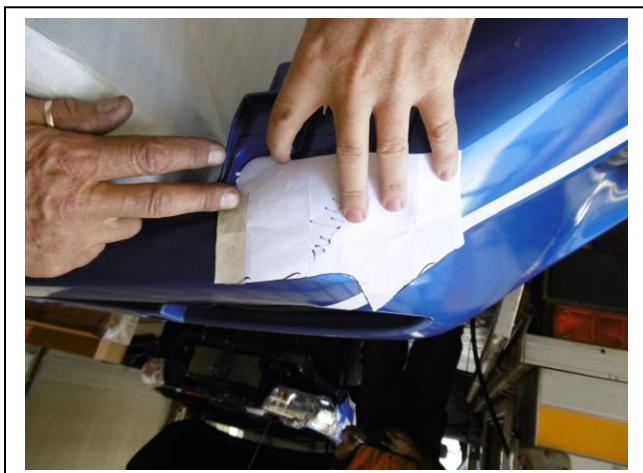
Figure 17. Liner trimmed to fit
