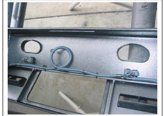
Figure 8: Wiring secured into bar. Parking sensor bar shown.
