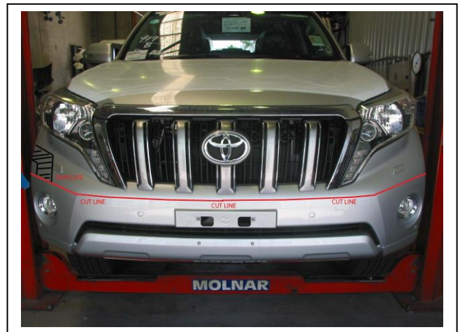
Figure 6: Cut line across front of vehicle.
