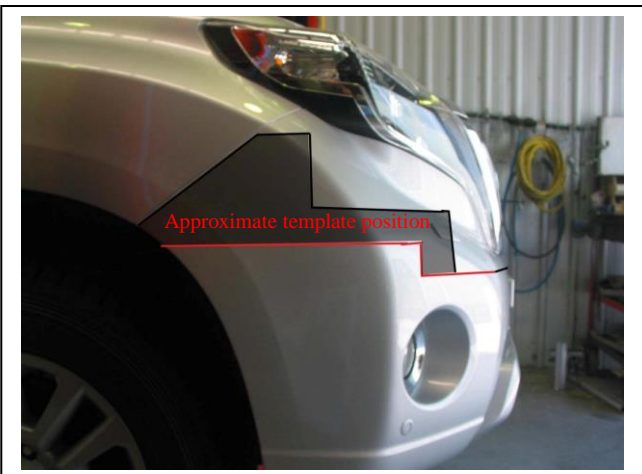
Figure 7: Cut line across front of vehicle.
