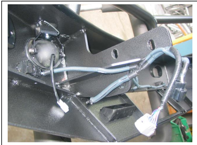
Figure 9: Wiring secured into bar. Parking sensor bar shown. NOTE wiring direction secured to
