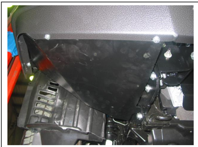
Figure 17: Passengers side under body guard
