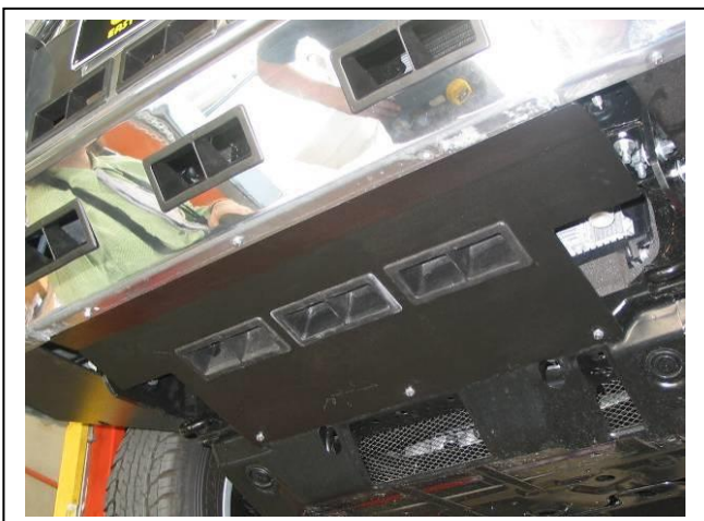
Figure 17: Centre under body guard fitted.
