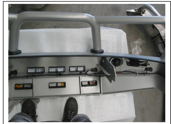
Figure 8: Parking sensor mounted into protection bar with secured wiring.
