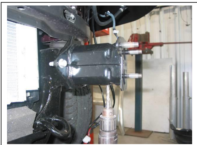
Figure 5: Drill holes to 10mm (3/8). Drill or die grind top to 18mm.
