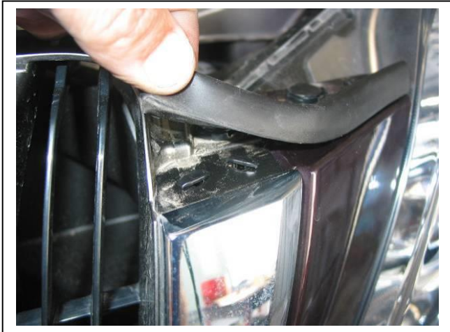
Figure 1: Rubber on top of grille. Take care during removal not to split rubber
