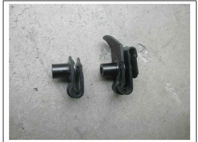
Figure 16: Cut down lower bumper clips for use on rear of inner guard
