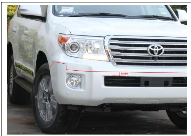
Figure 1: Approximate cut line on vehicle. Centre measurement is 55mm
