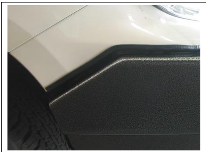
Figure 7: 3mm clip lock, trimmed to suit rear of cut
