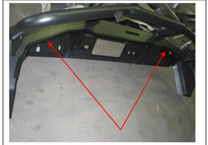
Figure 10: 6mm clip lock trim top view
