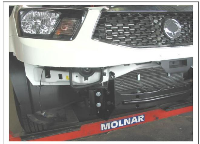
**Figure 1:** Front of completed bumper cut.
