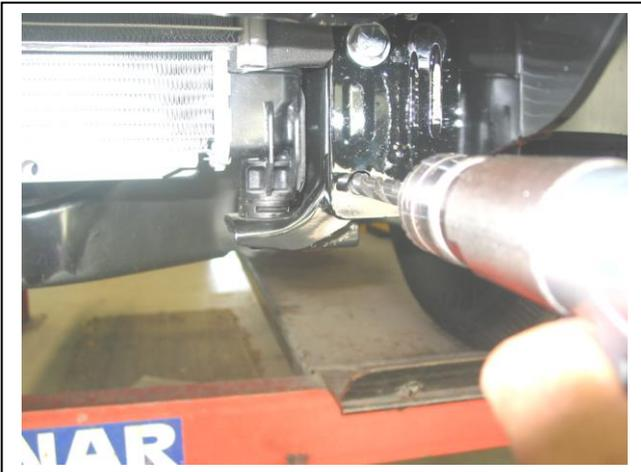
**Figure 4:** Drill lower mount to 13mm.
