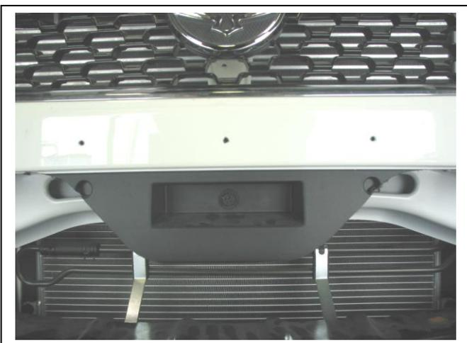
**Figure 2:** Retain recessed section and bolt in centre of bumper.
