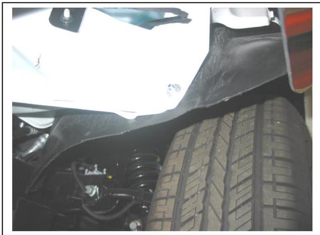
**Figure 12: Fitted and trimmed inner guard**
