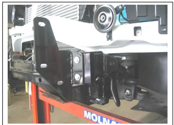
**Figure 3:** Steel mounting bracket installed to chassis rail.
