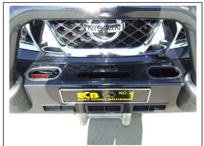
Figure 19: Inspection holes in top of Protection Bar
