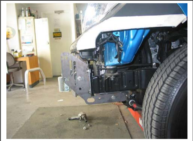
Figure 1: Place template to rear edge of bumper above crease line.
