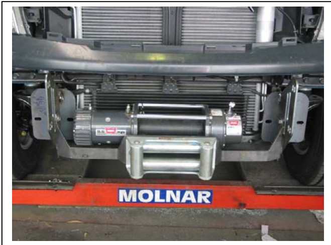
Figure 8: Fairlead rollers loosely attached to winch frame
