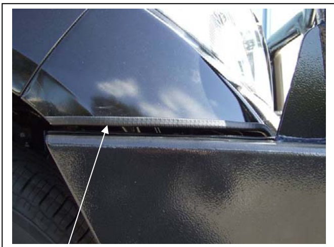
Figure 16: 3mm clip lock trim on outer cut edge of plastic bumper.
