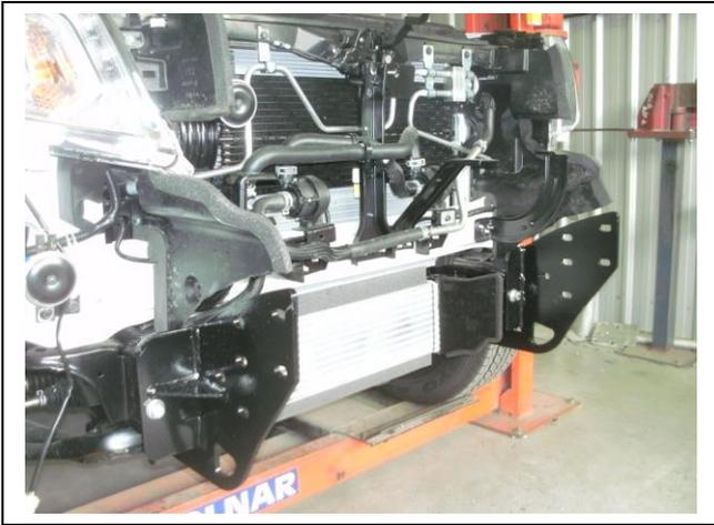
Figure 1: ECB steel mounts
