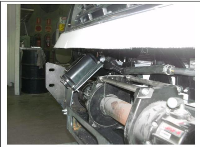
Figure 3: ECB winch mount with Mean Mother BOSS control box mounted
