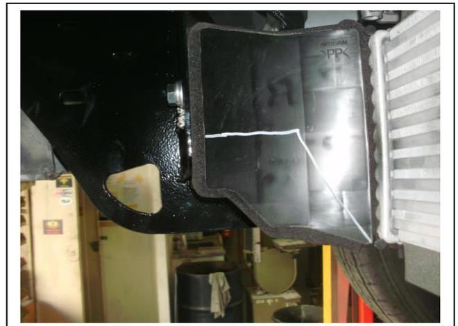
Figure 6: Intercooler air dam trim for under body guard fitment. Right hand side.
