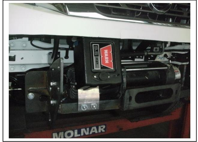
Figure 2: ECB winch mount with Warn 9.5 control box mounted
