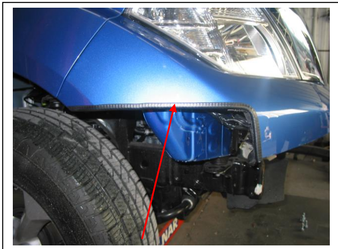
Figure 9: 3mm clip lock trim on outer cut edge of plastic bumper.
