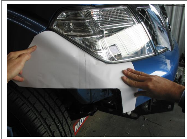
Figure 1: Align rear of template to plastic bumper / guard join. Mark and cut to shape.
