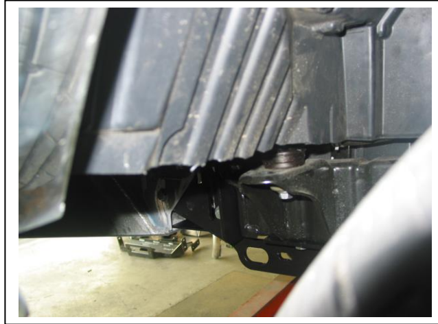
Figure 13: Trimmed under body guard, Passengers side shown
