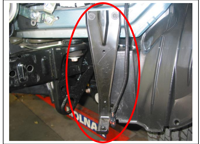
Figure 8: Remove side lower bumper supports.
