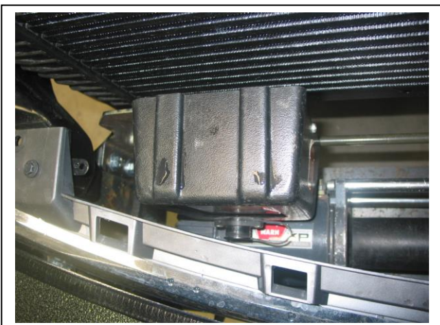
Figure 11: ECB control box mount
