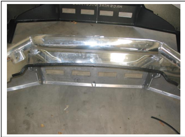
Figure 13: Centre clip lock trim fitted
