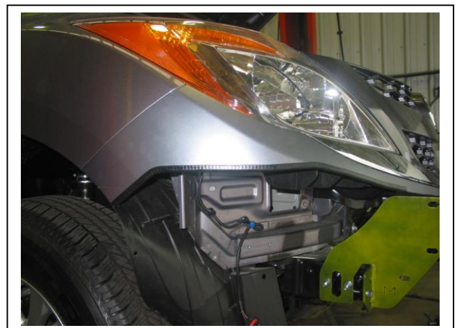
Figure 12: 3mm clip lock trim fitted to bumper cover
