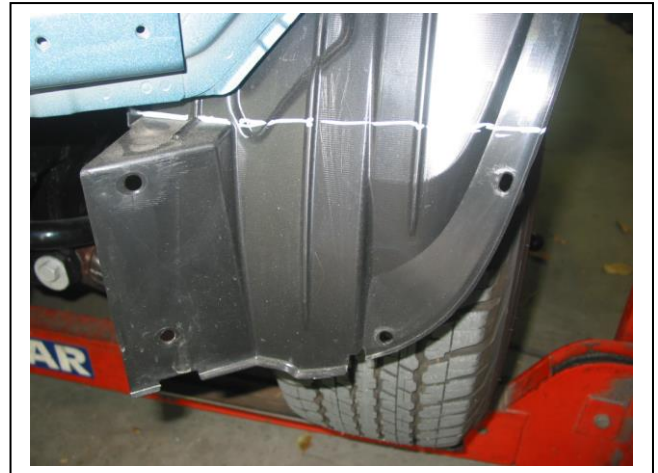
Figure 20: Approximate inner guard trim lines. Bumper removed for photo.
