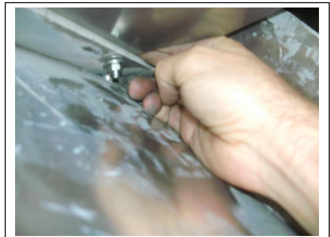
Figure 22: Placing bolt in from side of under body guard.
