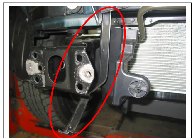
Figure 6: Remove center lower bumper supports
