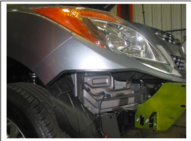
Figure 10: 3mm clip lock trim fitted to bumper cover
