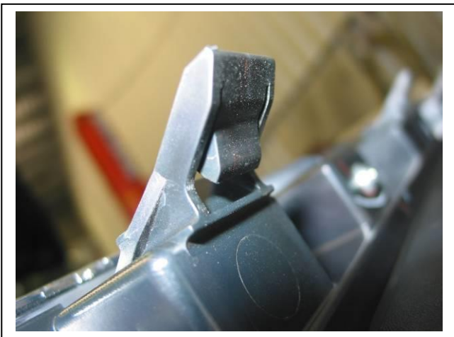
Figure 3: Clip on underside of grille
