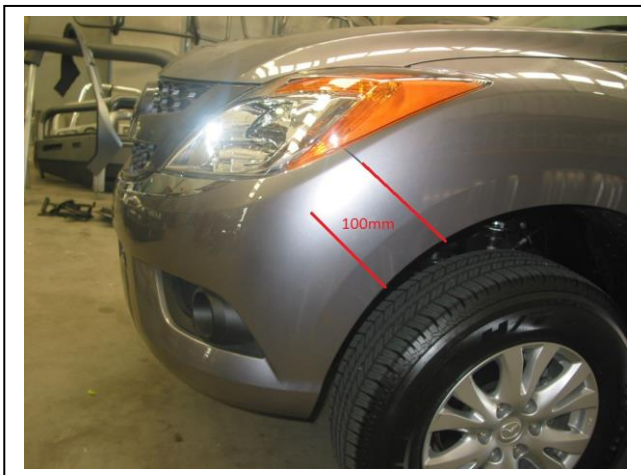
Figure 1: After masking vehicle, measure 100mm from guard join.
