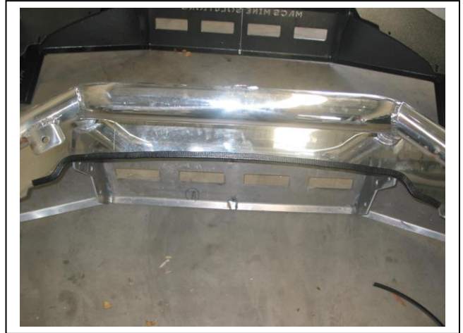
Figure 11: Clip lock trim fitted
