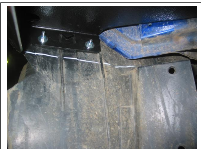
Figure 22: Cut line for inner guard.
