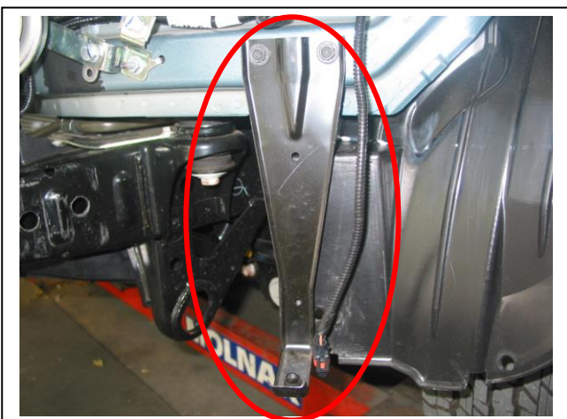
Figure 7: Remove side lower bumper supports. Use removed bolts to fit ECB inner guard supports
