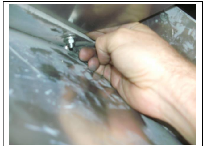
Figure 21: Placing bolt in from side of under body guard.
