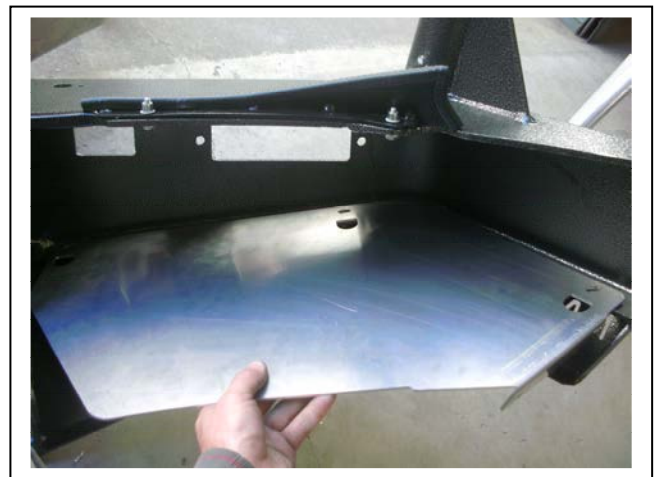
Figure 16: Placement of under body guard. Bumper removed for photo.
