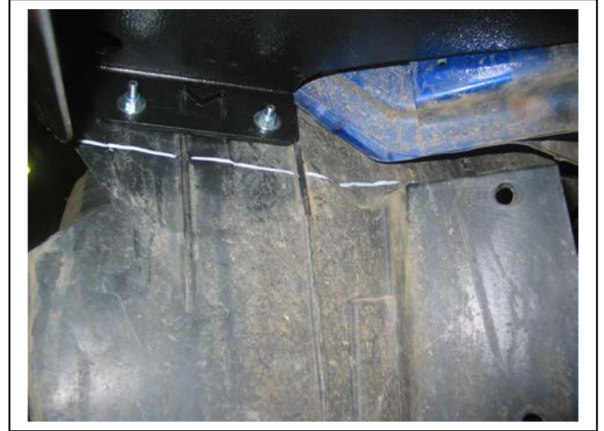
Figure 18: Cut line for inner guard.
