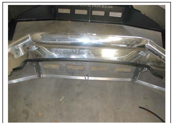
Figure 10: Clip lock trim fitted
