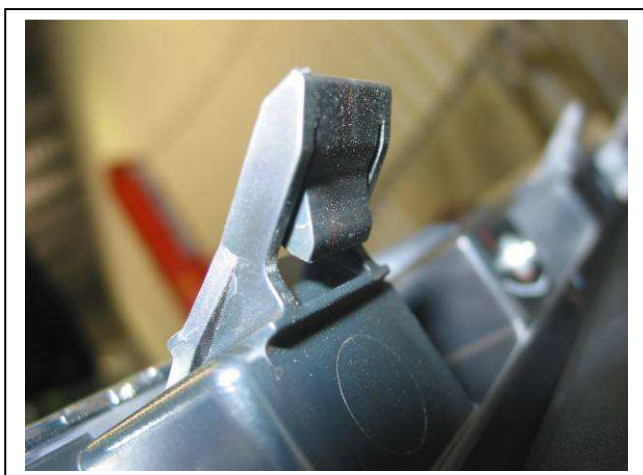
Figure 3: Clip on underside of grille
