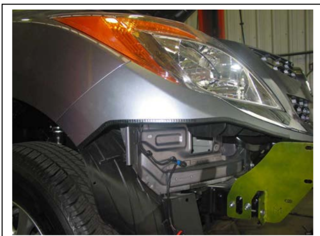
Figure 9: 3mm clip lock trim fitted to bumper cover
