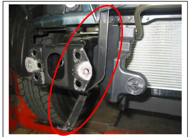
Figure 6: Remove center lower bumper supports
