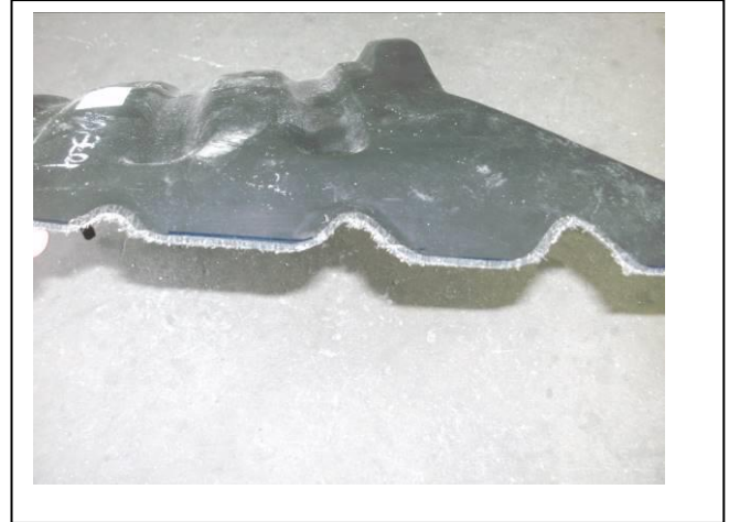
Figure 16: Liner looks like this after trimming
