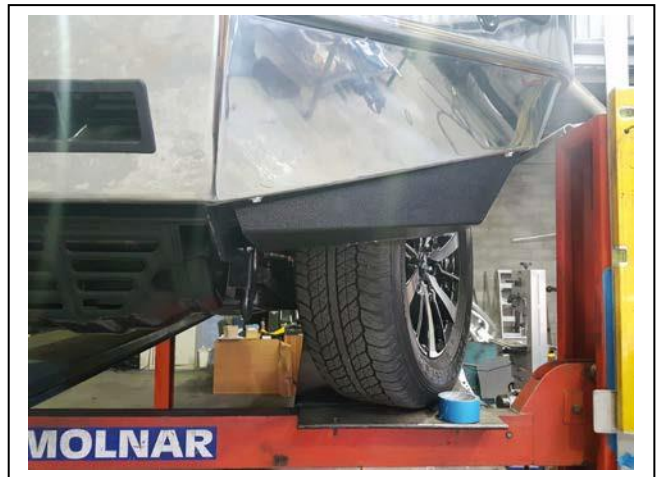
Figure 16: liner trimmed to fit guard
