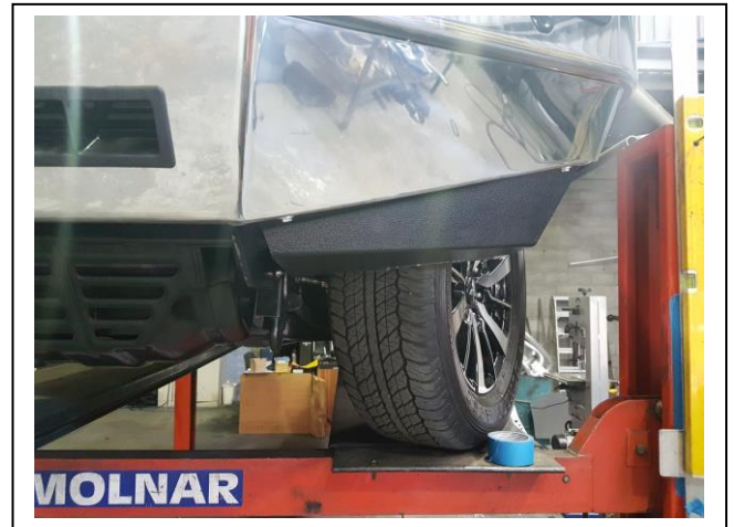
Figure 16: liner trimmed to fit guard
