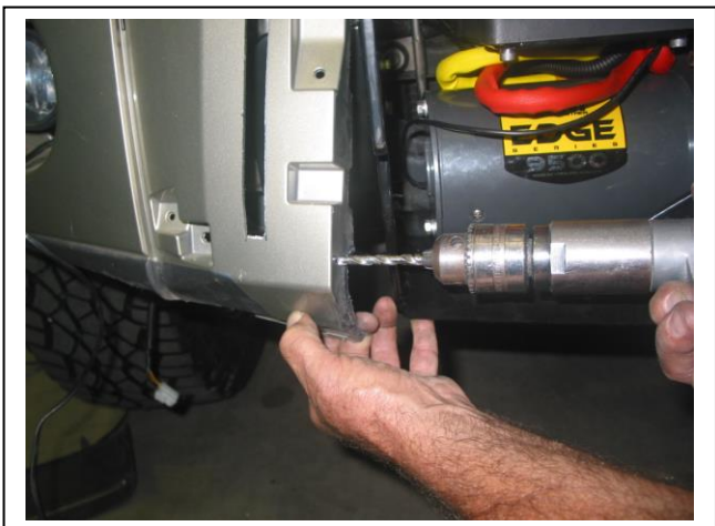
Figure 12: Drill marked hole to 6mm. insert 6mm alloy washer between bumper and winch frame when fitting.
