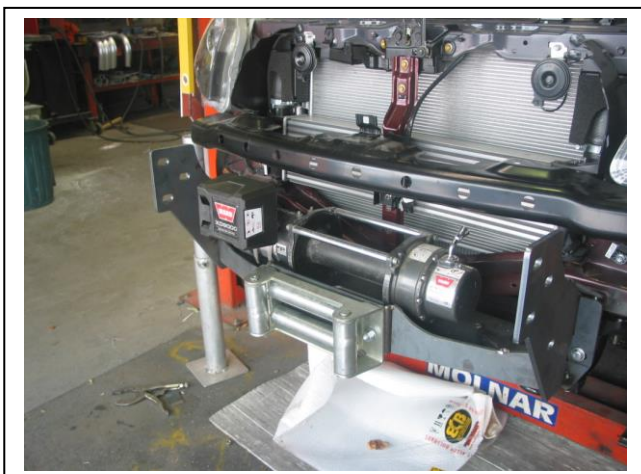
Figure 7: Warn XP9.5 fitted to winch frame.
