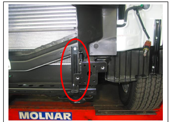
Figure 2: Passengers side inner bumper stiffener
