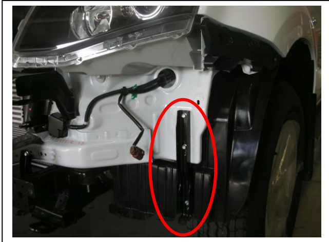
Figure 3: Passengers side outer bumper stiffener
