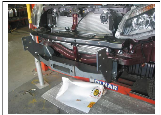
Figure 6: ECB winch frame.
