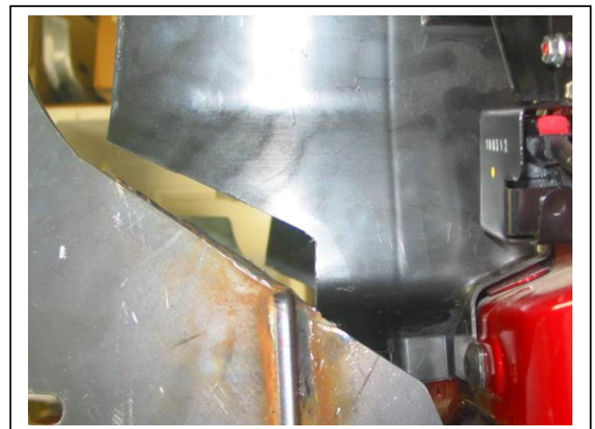
Figure 2: Trimmed area as seen behind mount. Caution: trim as little as possible.
