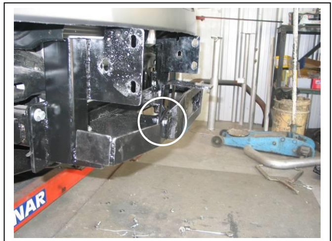
Figure 6: Control box mount fitted behind front face of winch frame
