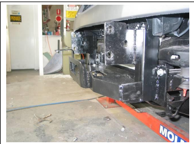
Figure 5: Winch mount fitted
