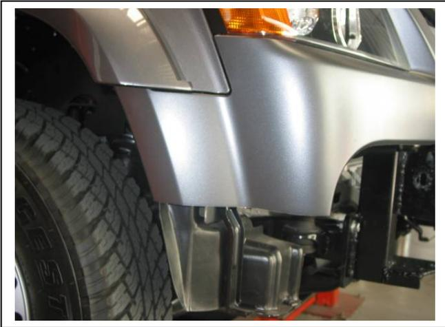
**Figure 1** Trim across join and around grille assembly.
