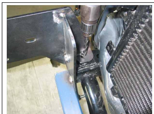
Figure 6: Drill hole in top of chassis rail to 10mm.
