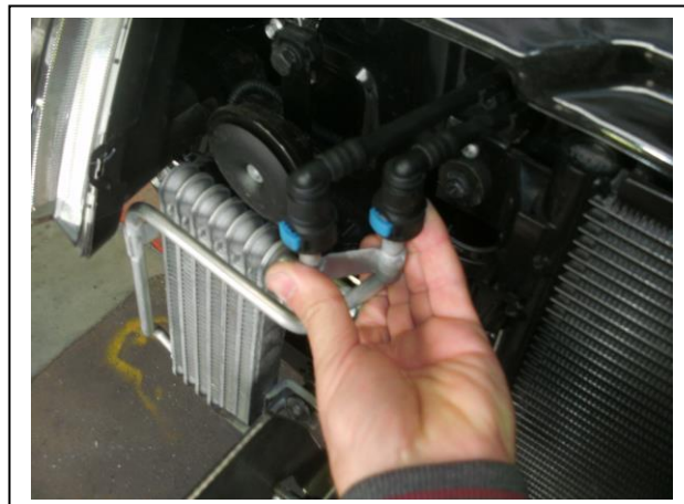
Figure 4: Adjusting oil lines to avoid them rubbing together.
