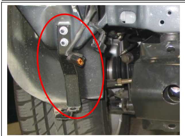
Figure 1: Side bumper support. Nuts are refitted to vehicle to support inner guard at a latter stage.
