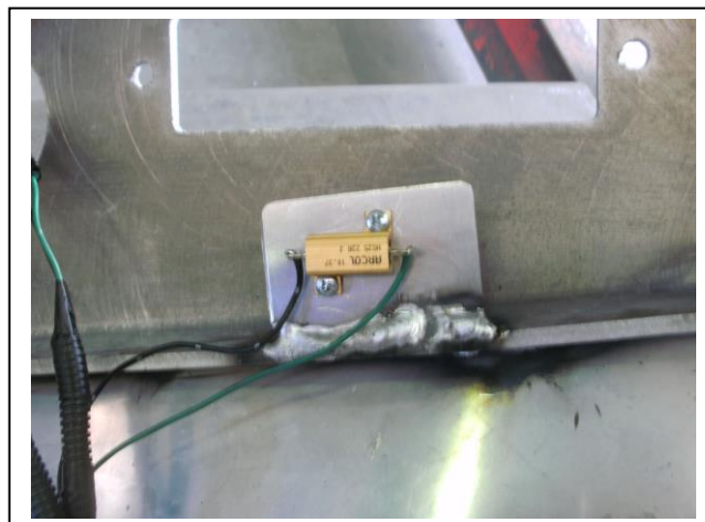
Figure 10: Placement of resistor on ECB protection bar. Caution: Load resistors get hot. Do not use plastic ties or attach to wiring. Keep all wiring clear.
